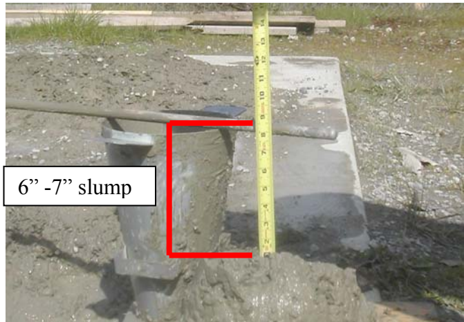
A 6" – 7" slump required an average of 20 pounds of pull force.
