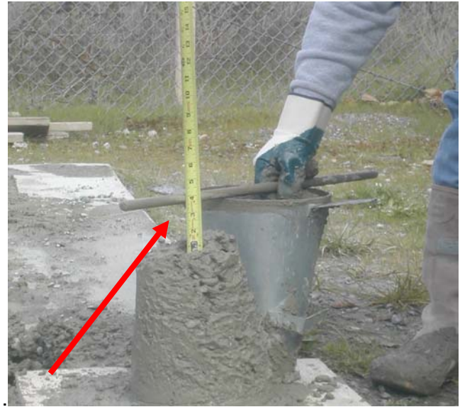
A 3" slump is measured here
