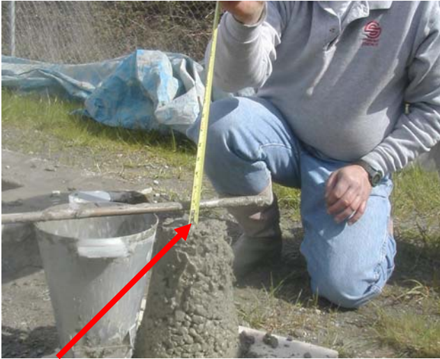
A 1" slump is measured here
